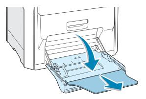
2 Load transparencies into the Multi-purpose Tray. They must be loaded with the print side downwards and the top with the white leading edge entering the printer first. Adjust the guide to fit the width of the transparencies.
